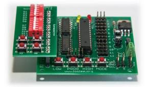
and set switch S1 OFF and S2-S4 ON. All other switches should be in the off position. Connect power as before.
